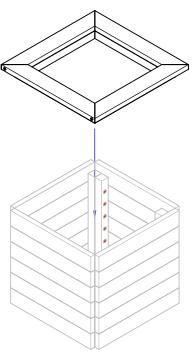
SLOT PRE-ASSEMBLED RIM ONTO PLANTER **ASSEMBLY**
